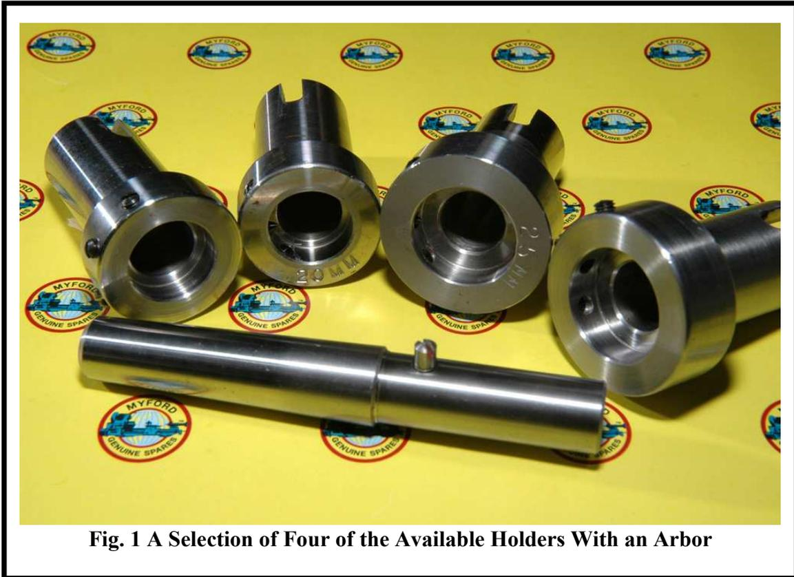
Myford Tailstock Die Holders, intended for thread forming from the tailstock, are available in six sizes. The individual sizes may be purchased separately in order to match the dies used by the customer, and an arbor is available which fits each of the holders and fits the 2 Morse Taper socket of the tailstock.
