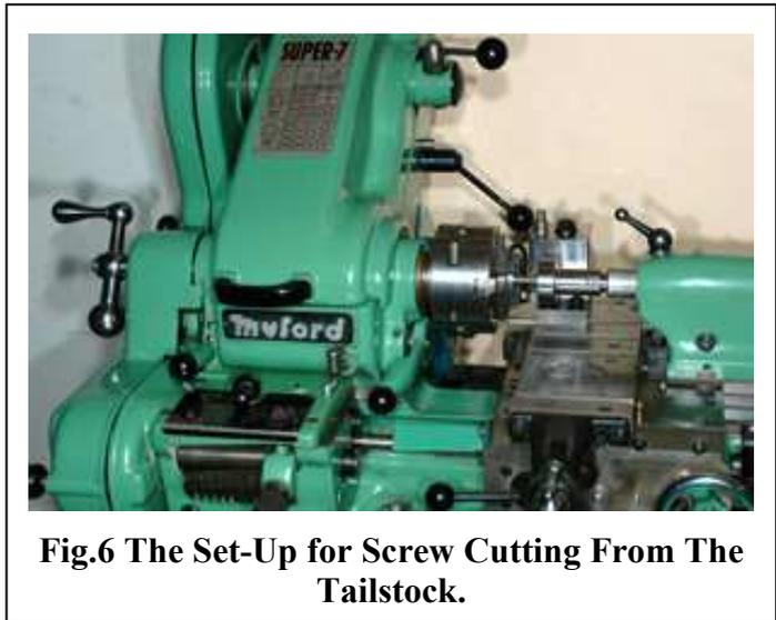
**Fig.6 The Set-Up for Screw Cutting From The Tailstock.**
