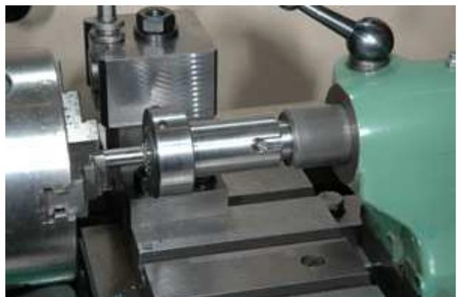
**Fig.5 Screw Cutting a Thread in the Tailstock**
