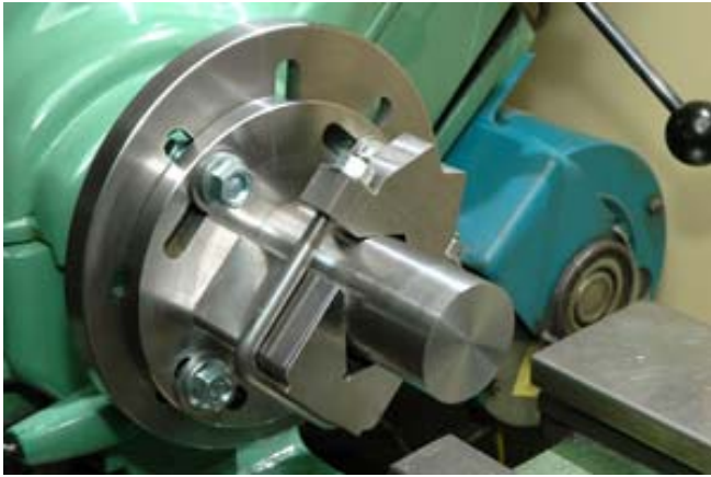
Photo.4 The Keats Plate is Attached Eccentrically on the Faceplate
