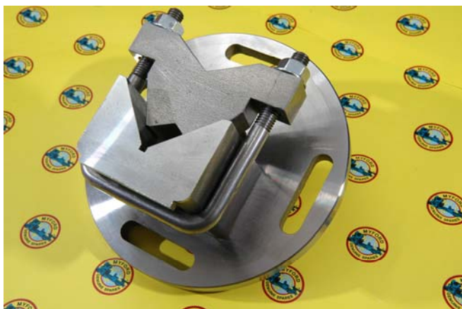
Photo.2 The Angle Plate Set Up For Smaller Diameter Items.
