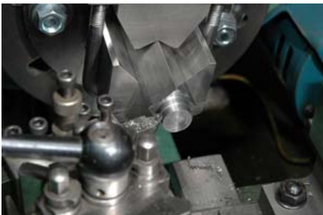
Photo.9 Turning a Square Bar
