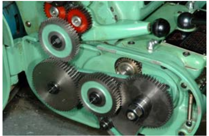
Fig. 6 The Gear Train for 1.25 mm Pitch
