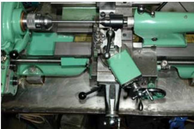
Fig. 11 Lathe Set-up for Screw Cutting
