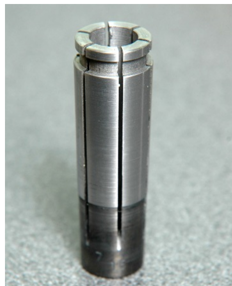
Photo. 14 A Finished Collet Ready For Use
