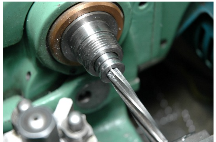
Photo. 11 Finishing a Collet Bore to Size
