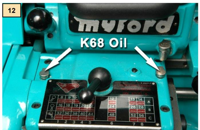
cient oil is required to eliminate the friction without splashing oil all over the surrounding areas. For lathes fitted with a Q.C. gearbox the gearbox requires lubrication entirely with K68 oil which is a gearbox oil.
