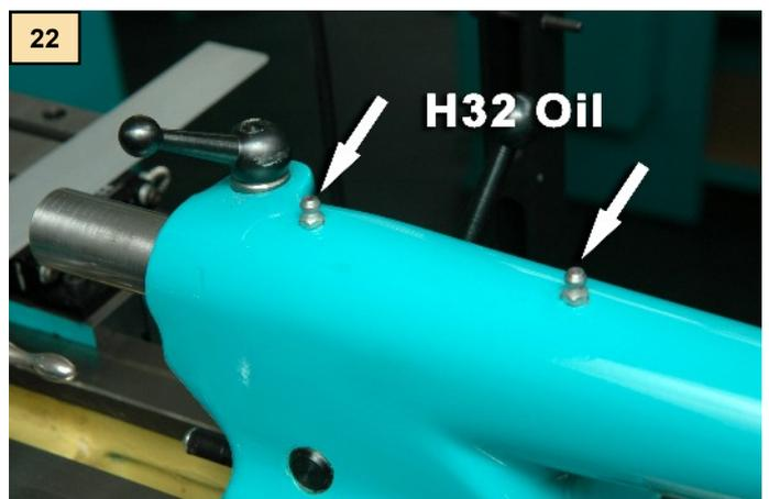
**Photo. 22** whilst the thrust bearing on the Super 7 is lubricated through the oil nipple in **Photo. 23** again with H32
