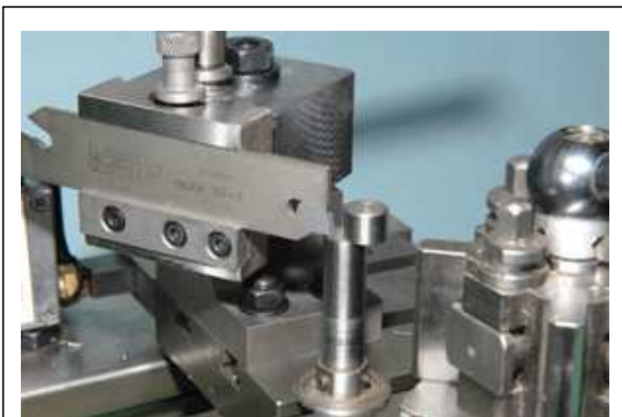
Fig.4 Adjusting the Height of the Blade .
