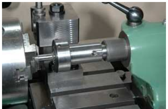
Fig.5 Screw Cutting a Thread in the Tailstock
