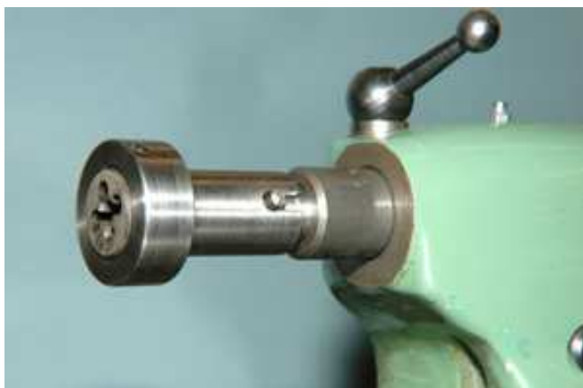
Fig.4 The Arbor and Die Holder Fitted to the Tailstock.
