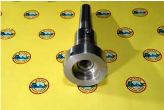
Fig.2 The Arbor is Bored Out For 32 mm. to Clear Long Threads
