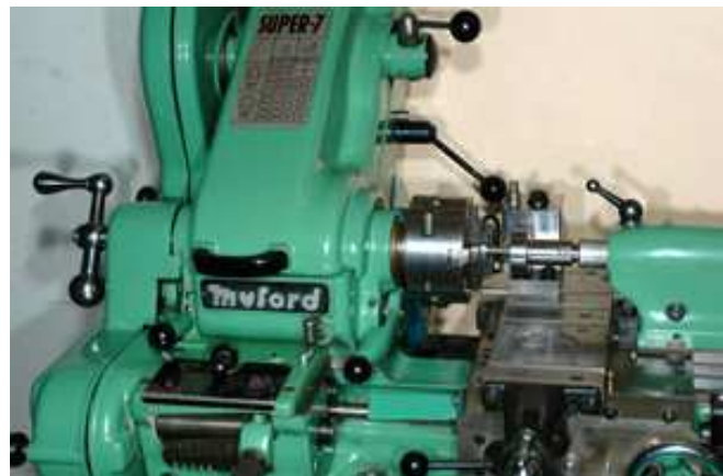
Fig.6 The Set-Up for Screw Cutting From The Tailstock.
