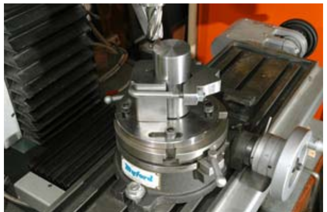
Photo.10 Preparing Work With The Keats Mounted on a Rotary Table
