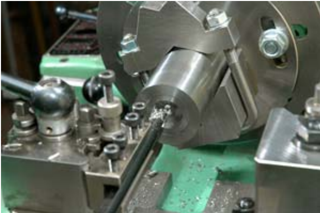
Photo.7 Boring The End of The Bar To Create a Bush
