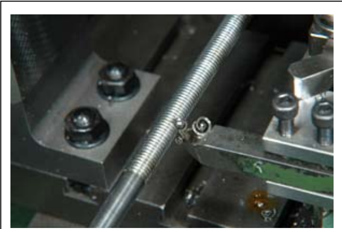
Fig. 13 Cutting The Thread
