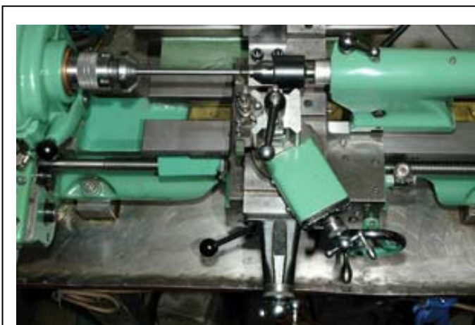
Fig. 11 Lathe Set-up for Screw Cutting
